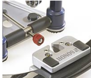
Smart Connect System The "Smart Connect" System ensures a quick and effortless attachment of the pedal with an adjustable ball clamp through a firm lever mechanism. A cylindrical axle connection neutralizes any possible tensions through different bass drum angle positions.
